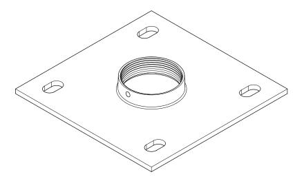
Thank you for choosing the VisionMount VMCA7 ceiling plate. The VMCA7 ceiling plate is designed to attach to an NPT 1-1/2 in. threaded pipe. The VMCA7 will support a maximum weight of 226.8 kg (500 lbs).
