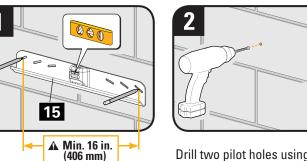
(8 mm) masonry drill bit. Position wall plate 15 at your desired height. Level, then
