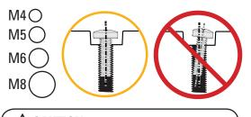
**CAUTION:** Verify thread engagment of the screw or spacer/screw combination in STEP 1-2. - Too short will not hold the TV — Too long will damage the TV
