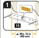
Position wall plate 15 at your desired height. Level, then mark the two hole locations.
