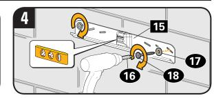
Install wall plate 15 with two washers 17 and screws 18, using bit 16. Securely tighten both screws 18
