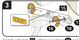
Install wall plate 15 with two washers 17 and screws 18, using bit 16.
