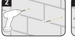
Drill two pilot holes using a 5/16 in.
