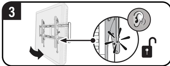
Press the bottom of your TV into the wall plate **10** until you hear the lock click, securing the TV in place.
