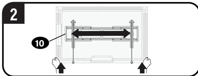
Lift your TV up then carefully reposition on the wall plate. The wall plate **10** has stops to limit lateral movement.
