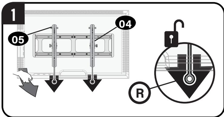
**To unlock your TV:** Pull down AND HOLD both release tabs **(R)** while gently pulling the bottom of the TV away from the wall.
