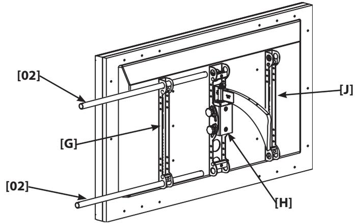
Attach the TV and arm assembly to the wall plate according to the instructions provided with the large VisionMount™ Full Motion Mount.
