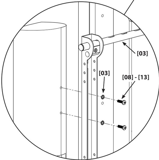
Determine the thread of the fastener required by threading each size fastener into the back of the speaker. Stop immediately if you encounter any resistance. Choose the correct thread size and fastener length for your speakers. If using M4 fasteners, [12] or [13], be sure to install the lock washer [20].
